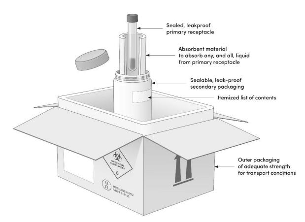
Figure 6: An example of triple packaging materials that may be used for Category A infectious substances
