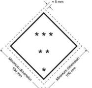
Figure 10: Template for hazard labels.
