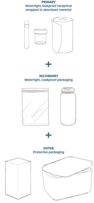
Figure 4: examples of basic triple packaging materials
