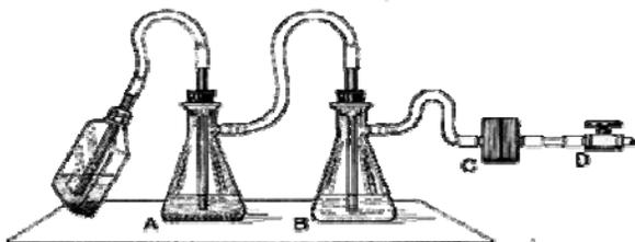
A suction flask is used to collect the contaminated fluids into a suitable decontamination solution. A second flask serves as a fluid overflow collection vessel and an in-line HEPA filter is used to protect the vacuum system from aerosolized microorganisms.
