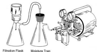
Improper trapping can allow vapor to be emitted from the exhaust of the vacuum system, resulting in either reentry into the laboratory and building or potential exposure to maintenance workers. Proper traps are important for both local pumps and building systems.
