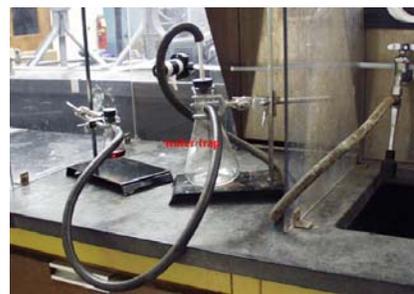
Only use this set-up if your solvent is non-volatile and non-hazardous, such as water. Methylene chloride and similar solvents will be drawn out of the flask and end up in the water being flushed down the drain through the water aspirator.
