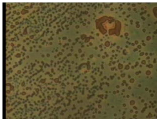
Figure 2: Dewetting Sample of PMMA/PS with .5% POSS
