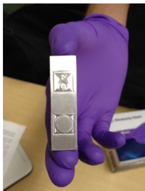
Figure 1: The aluminum mold used to create our backflow inhibitors.
