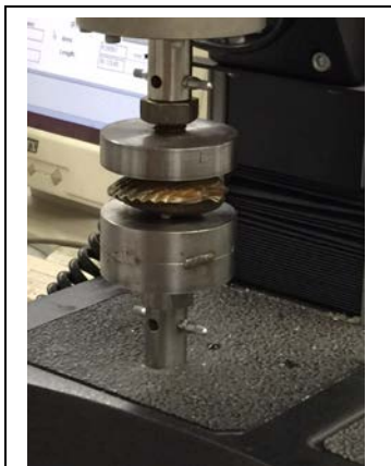
Figure 2. Scallop shell being compressed in the Instron machine.
