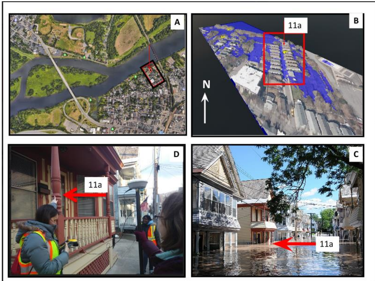
Figure 1: (A) Site 11a in Google Earth; (B) GlobalMapper simulation of the flood at site 11a using LiDAR data; (C) Flooding on Ingersoll Avenue in Schenectady, 2011; (D) Indicating high water mark at site.
