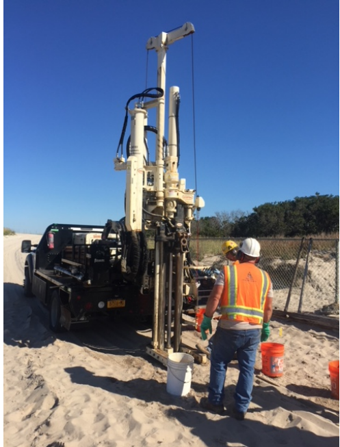
Figure 8. Geoprobe sampling at Robert Moses State Park, Oct. 2017.
