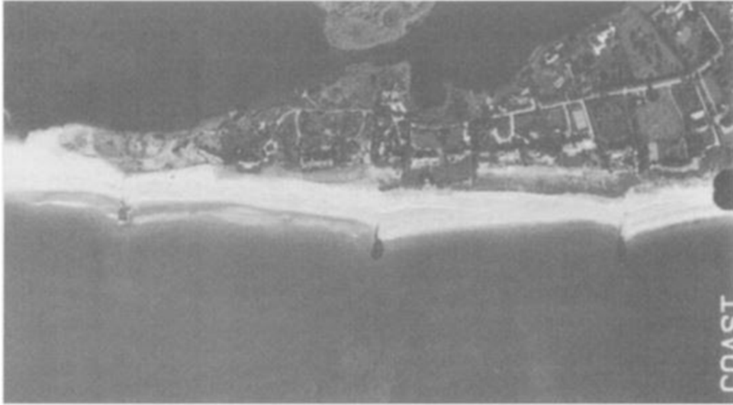
Figure 6. Geogica Pond groins in October, 1998 showing westward drift. Groins are 500 ft (152 m) apart.
