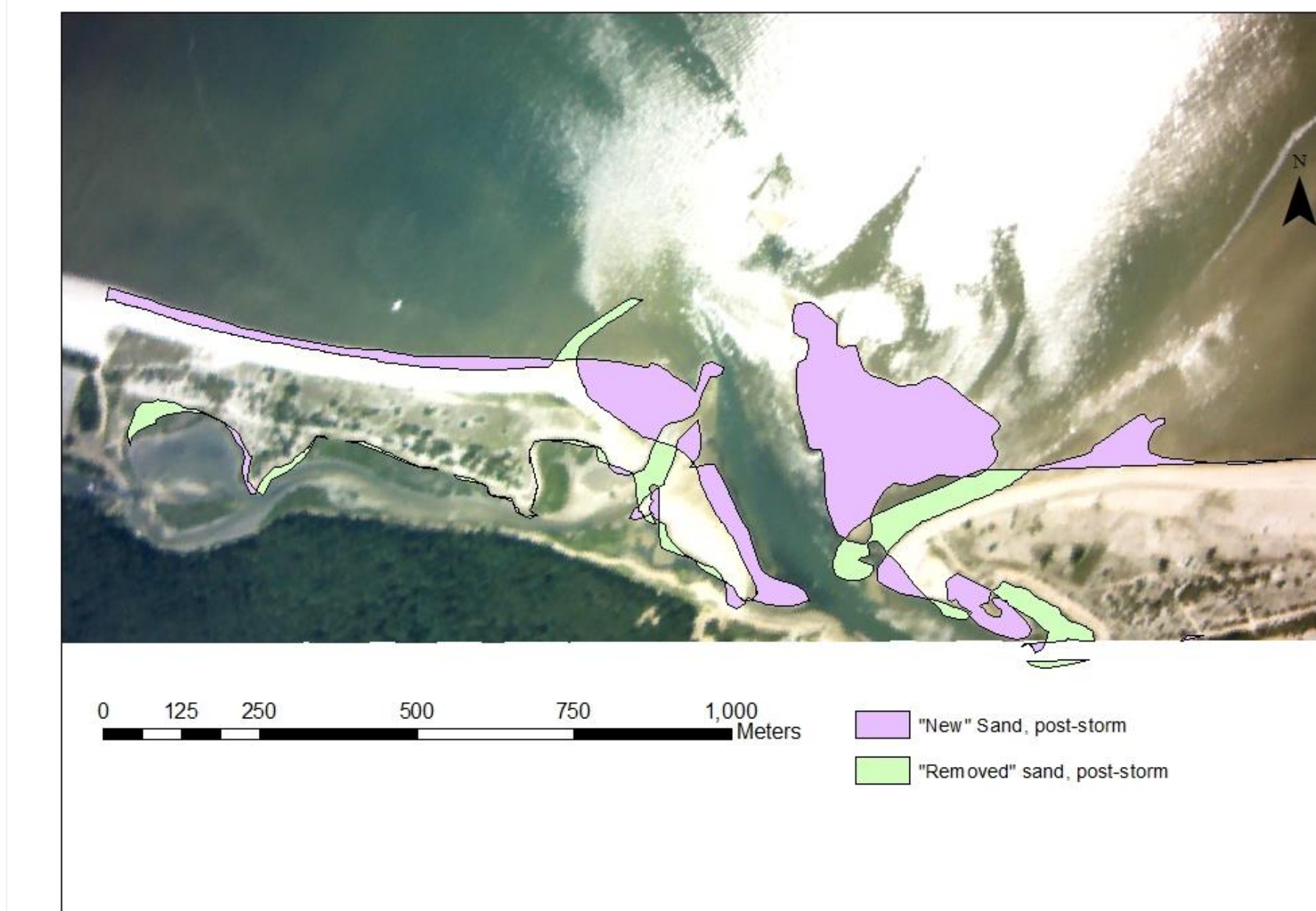
Figure 6. Estimated "new" and "removed" sand, as calculated using equation (2) and a conditional statement. Approximate area of "new" sand = 47,000 m 2 . Assuming sand has been deposited to a depth of 2 m, the estimated volume of new sand added from Hurricane Sandy is approximately 94,000 m 3 .
