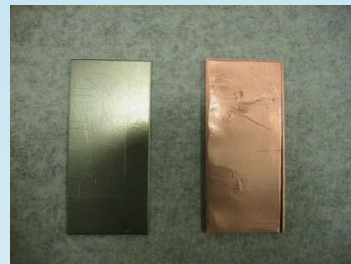
Corrosion Coupons Steel and Copper
